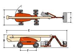
Platform: 36 x 96 in. (0.91 x 2.44 m) Side Entry 8 ft (2.44 m) JibPLUS\* Boom Selectable Capacity Envelope 180° Hydraulic Platform Rotator AC Receptacle in the Platform SkyPower\* Package
