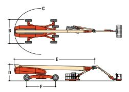
Platform 36 x 96 in. (.91 x 2.44 m) Side Entry Selectable Capacity Envelope
