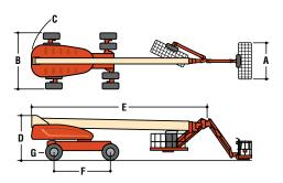
Platform: 36 x 96 in. (0.91 x 2.44 m) Side Entry 8 ft (2.44 m) JibPLUS\* Boom Selectable Capacity Envelope 180° Hydraulic Platform Rotator AC Receptacle in the Platform SkyPower\* Package
