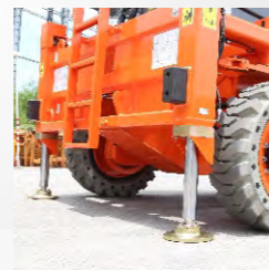
Self-leveling Hydraulic Outriggers
